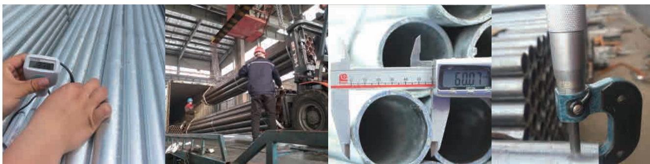
Zinc layer thickness
