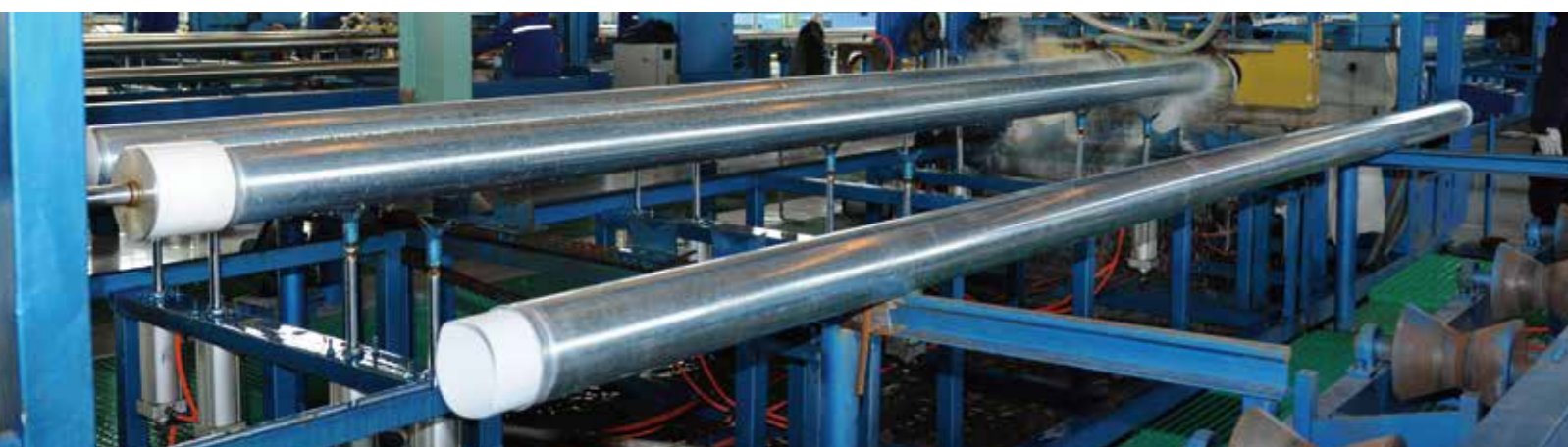
Steel Pipe of Lining Plastic Production Line
